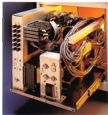
Pull-out drawer provides ready access to sophisticated electronics that drive precision transport
