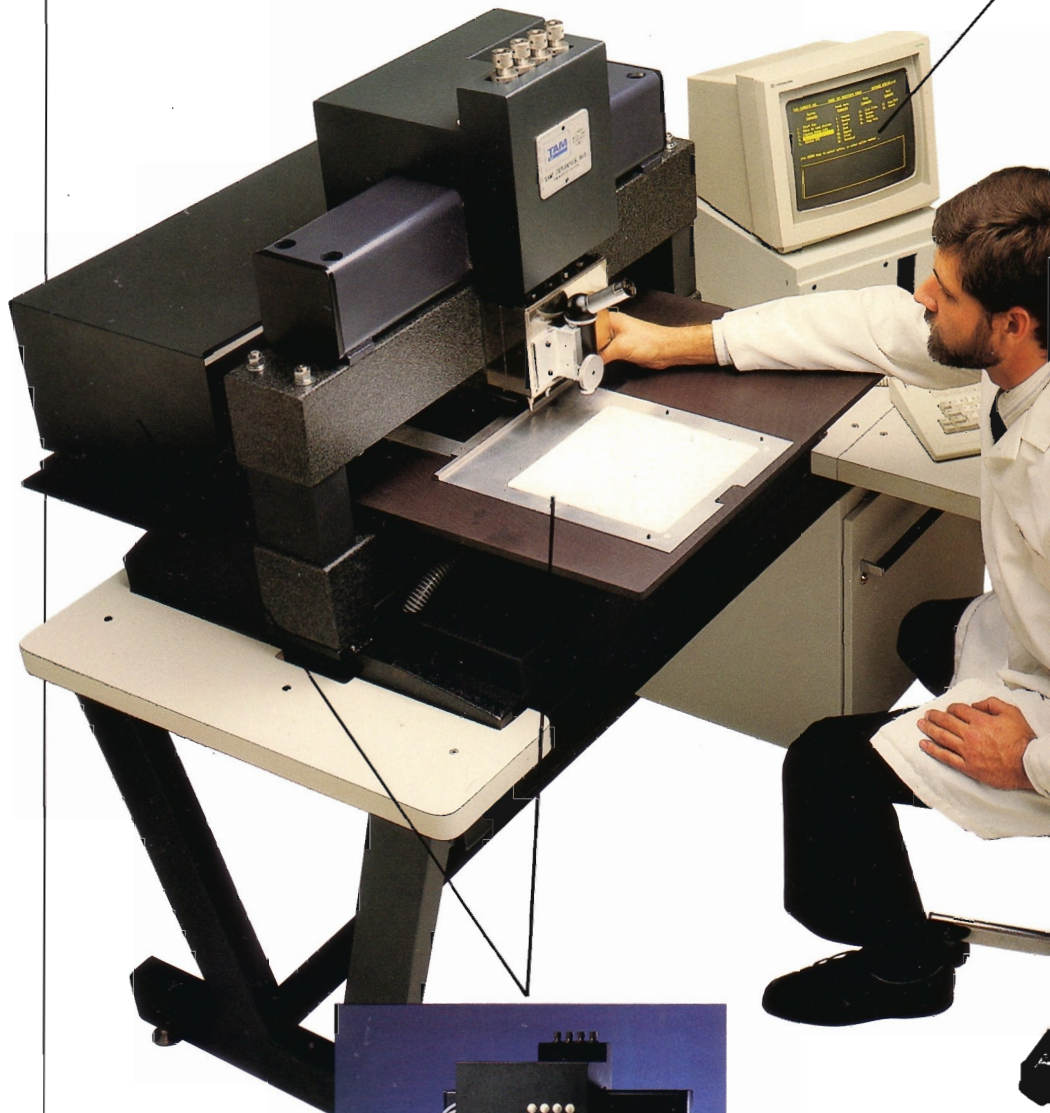
Linear stepper motors use precision technology originally developed for plotters to locate hole positions on substrates up to 100 in. sq.
